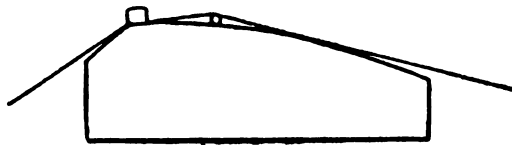
Fig. 6. Curved wooden bridge of tambura. Thread allows adjustable contact of string and bridge. (From Raman, 1922.)
